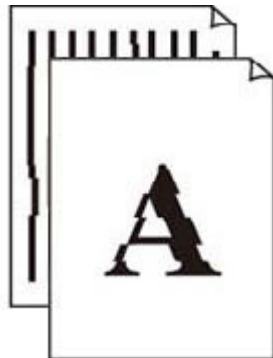
Lines Are Misaligned/Distorted
